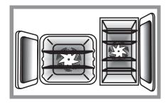
The fans in both ovens circulate hot air continuously, which means faster more even cooking.
